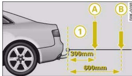
Fig. 234 Load distribution of equipment and accessories
