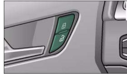
**Fig. 41 Driver's door: Central locking switch**
