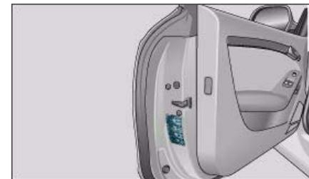
Fig. 261 Open driver's door (LHD vehicle) with sticker listing tyre inflation pressures
