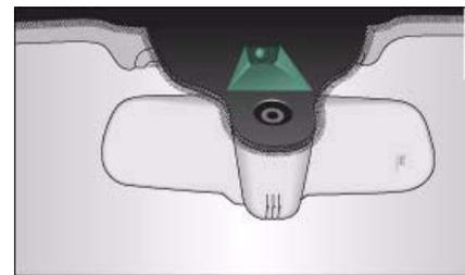
Fig. 159 Windscreen: Camera window for Audi lane assist
