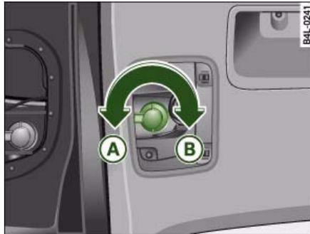
Fig. 287 Diagram: Bulb holder with a bayonet fastener
