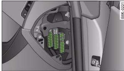
Fig. 285 Diagram of fuse box (left-hand drive vehicle)
