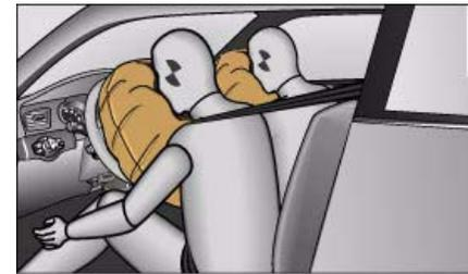
Fig. 216 Front airbags in inflated condition
