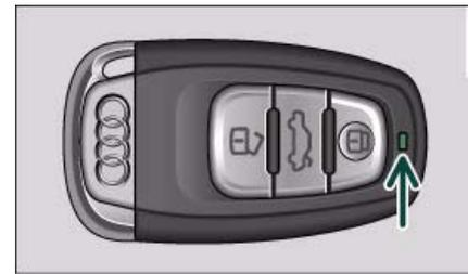
**Fig. 31 Indicator lamp on remote control key**
