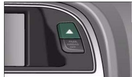
Fig. 60 Switch for hazard warning lights
