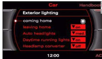
Fig. 56 Display: Exterior lighting
