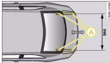
Fig. 246 Positions of securing points (from above)
