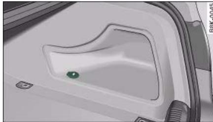
Fig. 98 Detail of the side trim in the luggage compartment: 12 Volt socket
