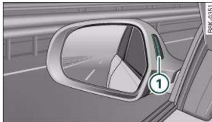
Fig. 164 Warning lamp on exterior mirror (driver's side)
