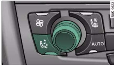
Fig. 117 Air distribution button and rotary control
