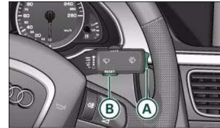
Fig. 20 Windscreen wiper lever: On-board computer controls
