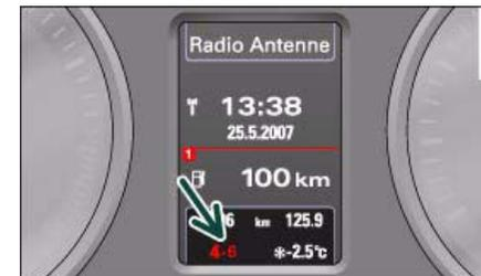
Fig. 11 Display: Gear-change indicator
