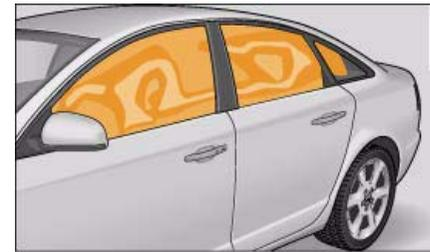
Fig. 221 Head-protection airbags in inflated condition
