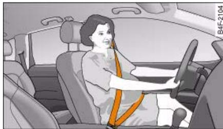
Fig. 211 Positioning seat belts during pregnancy
