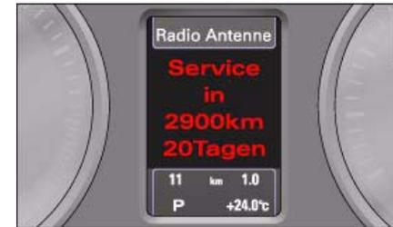
Fig. 15 Instrument cluster display: Service interval display
