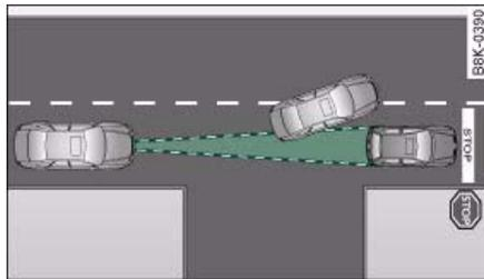
Fig. 155 Vehicle changing lane and vehicle stationary
