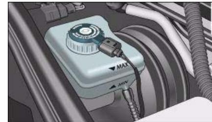
**Fig. 258 Engine compartment: Markings on brake fluid reservoir**
