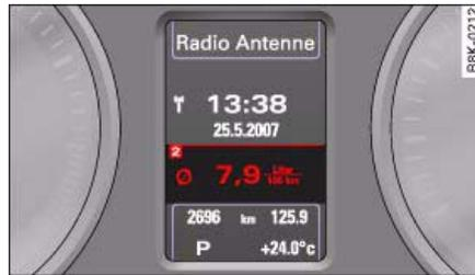
Fig. 18 On-board computer: Average fuel consumption
