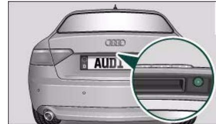
Fig. 191 Boot lid: Location of reversing camera
