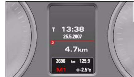
Fig. 181 Display: Manual gear selection (tiptronic mode)
