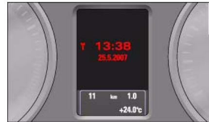
Fig. 4 Instrument cluster: Time and date display
