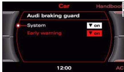
Fig. 157 Display: Audi braking guard
