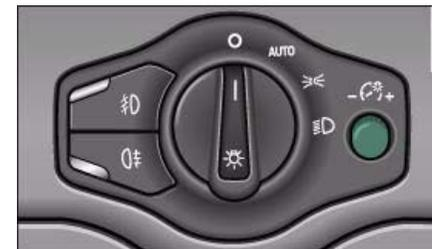
Fig. 57 Instrument lighting
