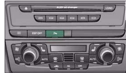
Fig. 185 Centre console: Parking aid switch
