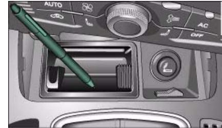
Fig. 184 Manual release of selector lever
