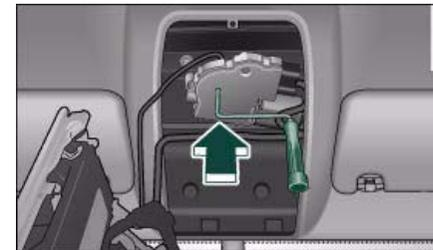
Fig. 53 Detail of headliner: Crank for manual operation
