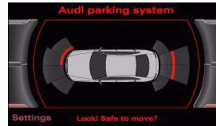
Fig. 186 Display: Graphical distance display
