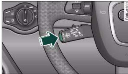
Fig. 139 Control lever for: Setting speed
