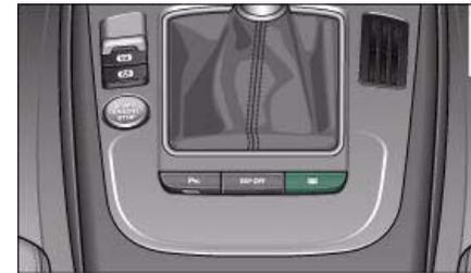
Fig. 66 Switch for sun blind
