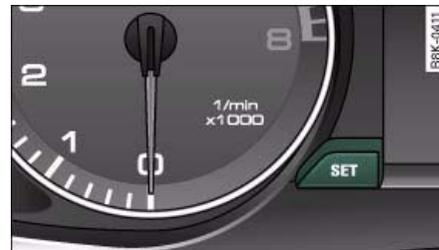
Fig. 22 Detail of the instrument cluster: SET button
