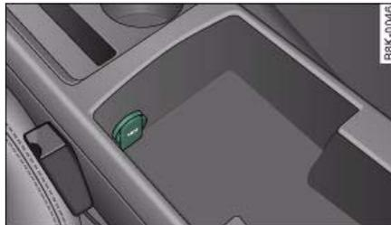
Fig. 99 Electrical socket in the centre console
