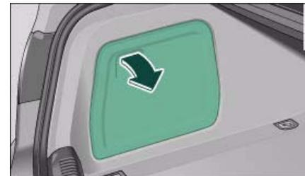
Fig. 86 Luggage compartment: Side trim with closed storage compartment ►
