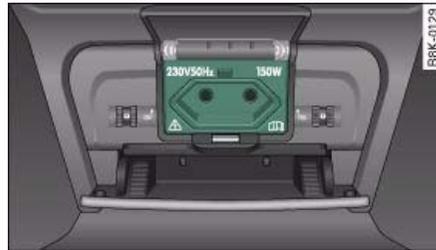
Fig. 100 Rear centre console: 230 Volt Euro socket
