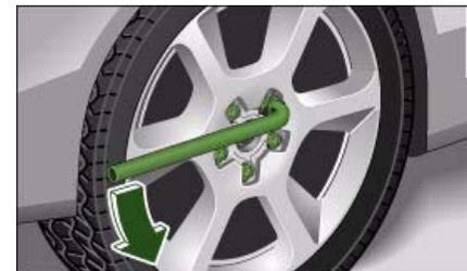
Fig. 272 Changing a wheel: Loosening wheel bolts
