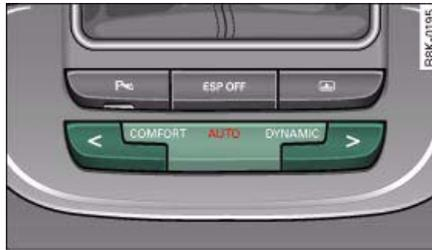
Fig. 174 Selector gate: Control for Audi drive select
