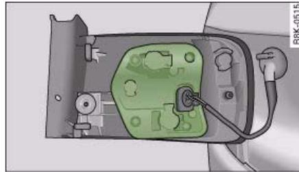
Fig. 304 Rear light, mounting plate is highlighted
