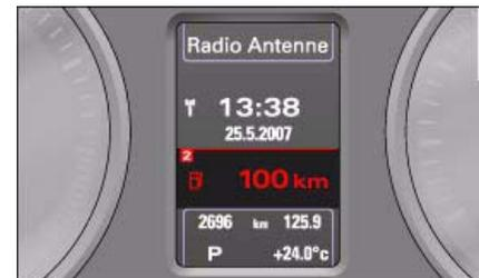
Fig. 17 On-board computer: Fuel range ►
