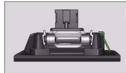
Fig. 311 Number plate light: Retaining element
