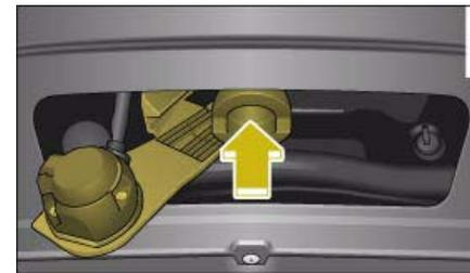
Fig. 240 Removable towing bracket: Inserting the ball joint
