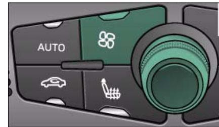
Fig. 106 Blower button and rotary control
