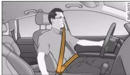
Fig. 208 Positioning of head restraints and seat belts
