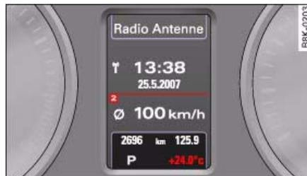
Fig. 10 Display: Outside temperature
