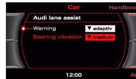
Fig. 162 Display: Setting time of warning and steering vibration
