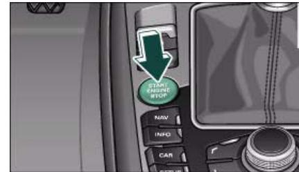
Fig. 131 Audi advanced key: START ENGINE STOP button
