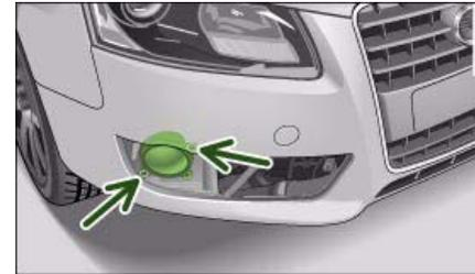
Fig. 299 Screws securing fog light
