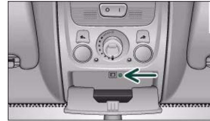
Fig. 52 Detail of headliner: Unscrewing the light housing
