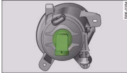
Fig. 300 Front fog light: Bulb holder is highlighted
