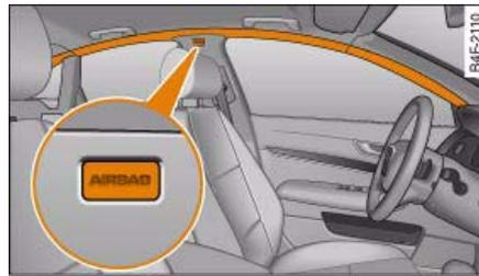
Fig. 220 Location of head-protection airbags above the doors
