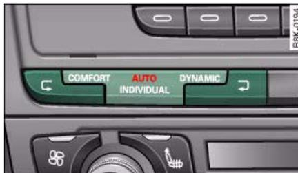
Fig. 175 Centre console: Control for Audi drive select
