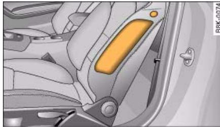
Fig. 218 Location of side airbag in driver's seat
