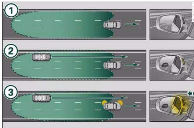
Fig. 167 side assist: Vehicles approaching rapidly from behind
