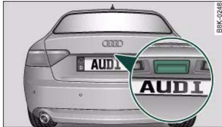
Fig. 46 Release catch on the boot lid
