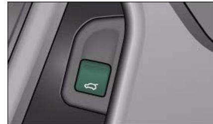
Fig. 45 Driver's door: Unlocking the boot lid ▶
