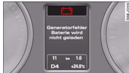
Fig. 25 Display: Symbol for serious malfunction
