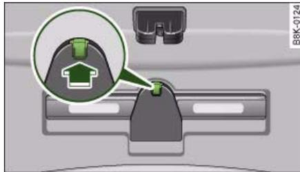
Fig. 264 Warning triangle fitted inside boot lid
