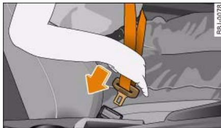
Fig. 209 Driver's seat: Belt buckle and latch plate
