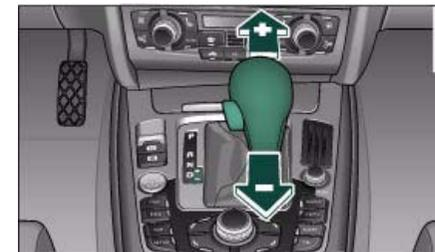
Fig. 180 Centre console: Manual gear selection (tiptronic mode)
