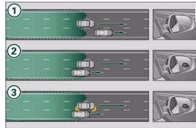
Fig. 170 side assist: Other vehicles being overtaken rapidly
