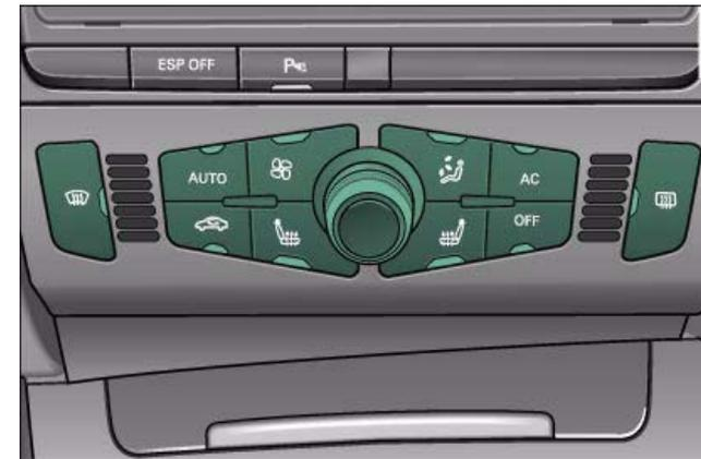
**Fig. 103 Controls for deluxe automatic air conditioner**
