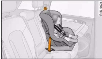
Fig. 227 A category 1 forward-facing child seat fitted on the rear seat
