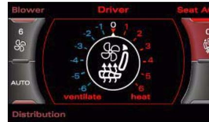
Fig. 128 Display: Seat heating/ventilation
