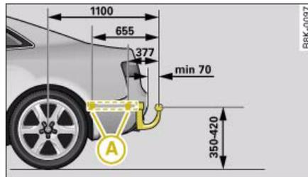
Fig. 245 Positions of securing points (side view)
