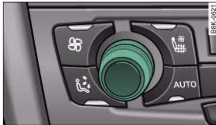
Fig. 113 Rotary control for temperature selection
