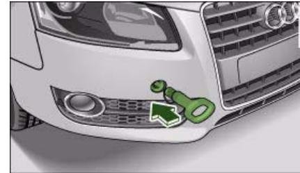
Fig. 281 Front bumper: Fitting the towing eye
