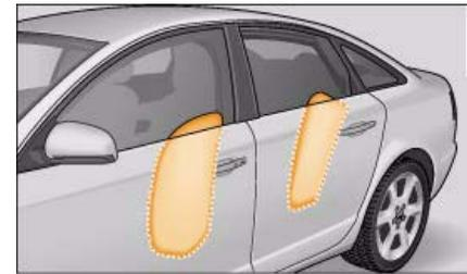
Fig. 219 Side airbags in inflated condition
