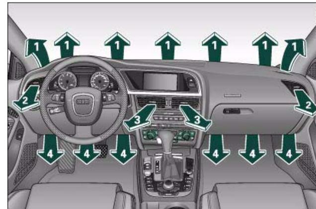
Fig. 119 Dashboard: Location of air outlets
